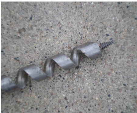
A ship auger bit will remove wood chips better than a wood drill bit.
